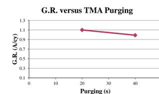
The growth rate decrease by 10% when lengthening the purging time of TMA from 20s to 40s. This is due to an increased removal of excessive surface-adsorbed chemicals.
