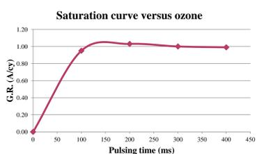
Saturation studies shows that the growth saturates at 100 ms dosing of ozone. In subsequent runs a 200 ms ozone dose was used.
