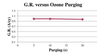
The growth rate did not change when lengthening the purging time of ozone from 5s to 20s. Normally 5s was used. This is much shorter than purging of water at the same 60 C.
