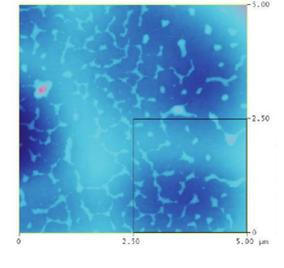
The rms for ALD TiO<sub>2</sub> at 150C is 6 nm for 50nm film
