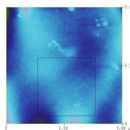
The rms for ALD TiO<sub>2</sub> at 100C is 2nm for 50nm film
