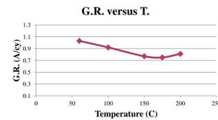
Growth rate versus temperature study shows that growth rate stabilized at the window of 150 C and higher. At temperatures below 150C the growth rate increased with lowering temperature. This is due to the insufficient removal of excessive surface-adsorbed material, most probably oxygen
