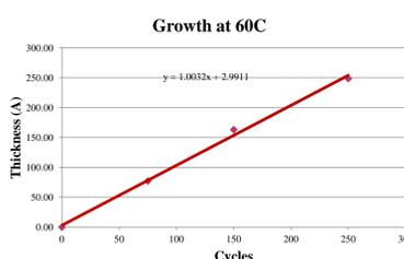
The linear growth shows the typical ALD behavior of LT Al<sub>2</sub>O<sub>3</sub> process with growth rate of 1.0A/cy.
