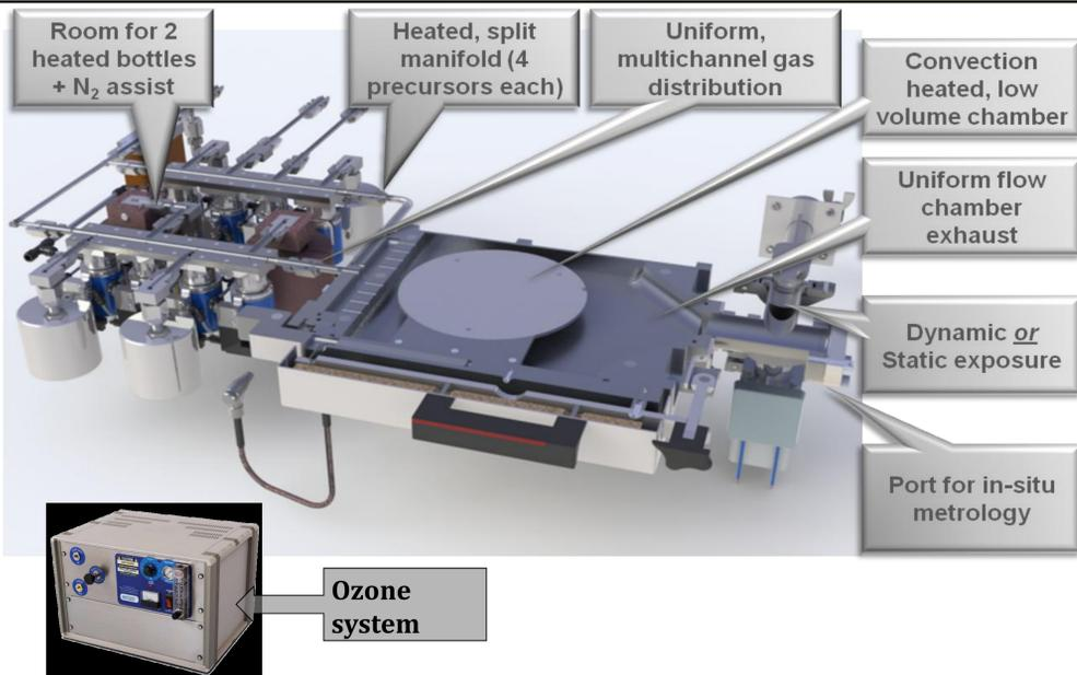
GEMStar-8 system is designed for extreme surface area, high aspect ratio structures: Multi-channel precursor delivery system isolates & distributes precursors combine with a tapered exhaust to provide exceptional nanofilm uniformity.
