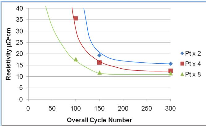
Resistivity as a function of cycle number for different Pt pulses all at 70 °C – AR ~ 25:1 cycles (~7.5nm) and uniform physically and electrically to AR >150:1 (see below).
