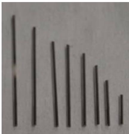
One way we examine the growth characteristics of conductors is by growing the films in fused silica capillary tubes and measuring the resistance from end to end through the interior of the tube after ALD. The image to the left shows an experiment where a Pt film was conformal over the first 7 tubes and doesn't quite connect with the 8<sup>th</sup> tube (far left). Electroding the tubes and then measuring the resistance produces a plot
