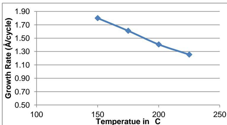
Figure 4 - GR of ZnO vs Temperature
