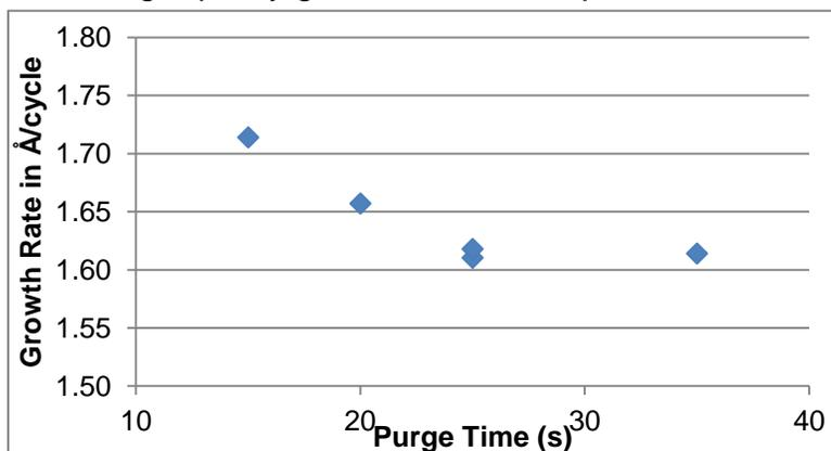
Figure 3 - ZnO growth rate as a function of DEZ purge time at 175C
