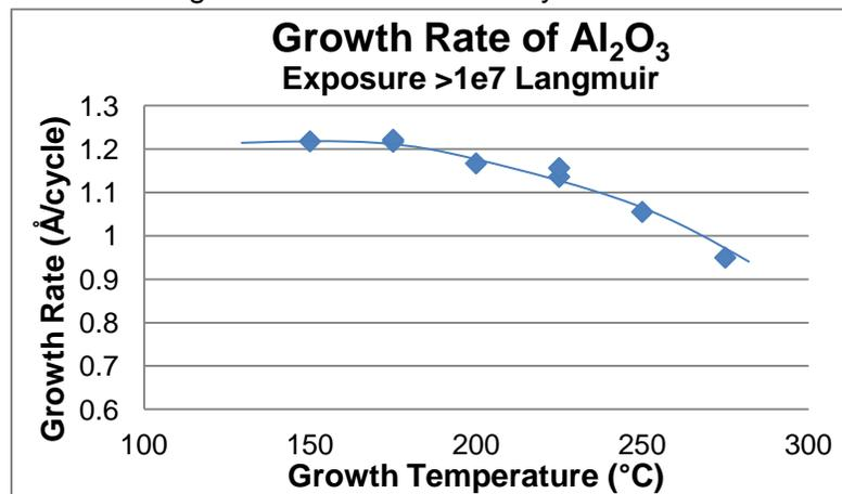
Figure 1 - Growth rate of Al<sub>2</sub>O<sub>3</sub> as a function of temperature in GemStar
