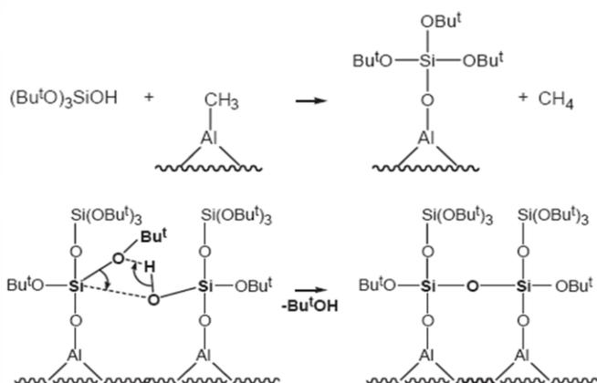
Figure 5 - Catalytic silica mechanism
