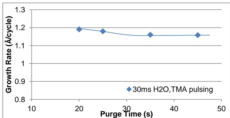
Figure 2- Growth rate as a function of Purge time at 200C
